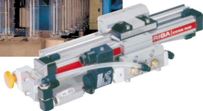
Macro-component used in a plastic blow-moulding machine - for forming plastic bottles The drive moves a filler neck which shapes the PET bottle with high pressure air (40 bar) in the forming die
