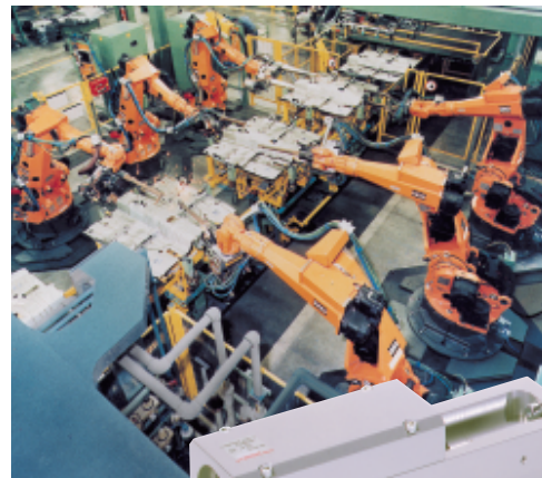
Pneumatic feed unit for positioning welding heads in automatic welding devices
